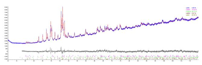
Fig. 3. X-ray diffraction pattern of the as-cast alloy 29La–71Ni. Red curve: pattern calculated from Rietveld Refinement; blue curve: experimental pattern; grey curve, bottom: difference curve.
