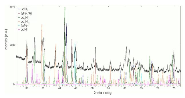
Fig. 9. X-ray diffraction pattern of the as-cast alloy 25Fe-55Ni-20La (#11).
