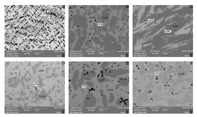
Fig. 8. Microstructure of annealed at subsolidus temperatures alloys of the La-Ni-Fe system:
