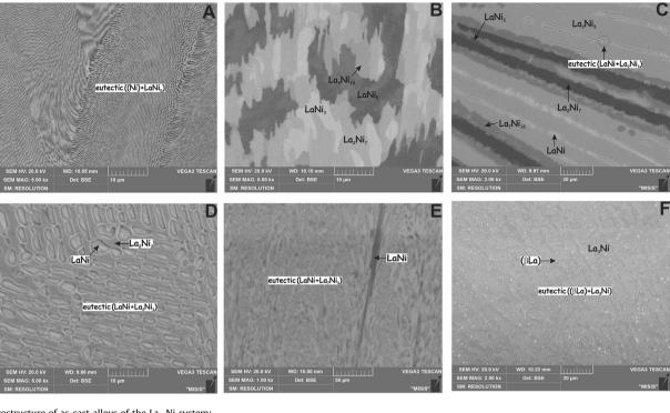
Fig. 2. Microstructure of as-cast alloys of the La–Ni system: a - 8.5La-91.5Ni,  $\times$  5000, eutectic ((Ni) + LaNi<sub>5</sub>);
