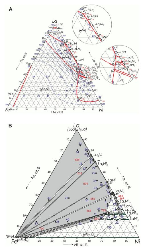
Fig. 6. Liquidus (a) and solidus (b) projections and the melting diagram (c) of the La–Ni–Fe system:  $\bigcirc$  – composition of sample,  $\bigcirc$  – two-phase sample,  $\spadesuit$  – three-phase sample,  $\bigtriangleup$  and  $\blacktriangle$  – EPMA data of as-cast and annealed alloys, respectively.
