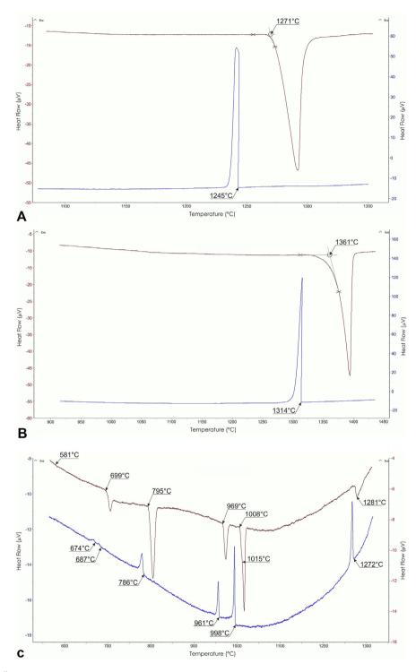
Fig. 1. DTA curve for La-Ni alloys:
