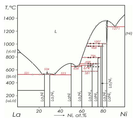
Fig. 5. Phase diagram of La−Ni system: △, ▲ − DTA data of as-cast and annealed alloys, respectively; ● − two-phase sample.
