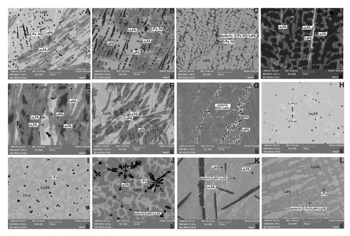
Fig. 7. Microstructure of as-cast alloys of the La-Ni-Fe system:
